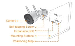
Step1 Drill screw holes on the mounting surface as the positioning map shows, and then put in the expansion bolts.
